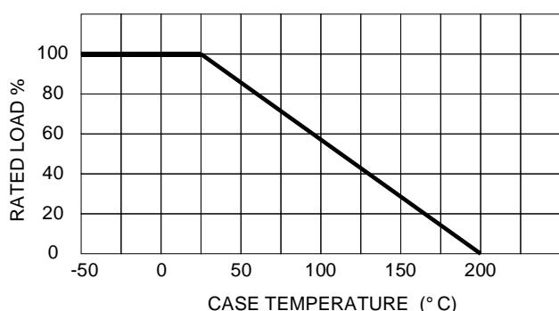
The case temperature is to be used for purposes of establishing the maximum applied power. The case temperature measurement is made with the thermocouple contacting the bottom insulated mounting surface of the package (center of bottom surface), the device mounted on a heat sink, thermal grease applied at a mounting torque of up to 90 N·m (8 in-lbs) max.
